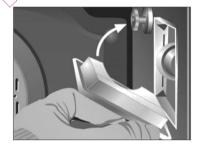
The replacement bulb must be temperature resistant to 300 °C. These can be ordered from the Technical Service Department.
