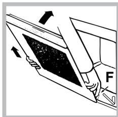
3. (with glass panel fitted to the inside of the door) Grip the door on the two outer sides and close it approximately half way. Unlock the door by pressing on the clamps F, then pull the door towards you, lifting it out of its slot
