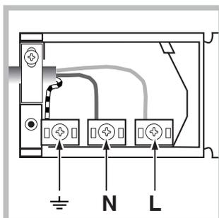
2. Install the power supply cable by loosening the cable clamp screw and the three wire contact screws L-N-. Connect the wires to the corresponding terminals: the Blue wire to the terminal marked (N), the Brown wire to
