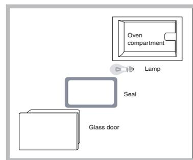
1. Remove the glass cover using a screwdriver.
