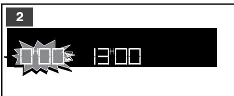
The display stops flashing after a few seconds and the timer starts to run, counting down the time in seconds.
