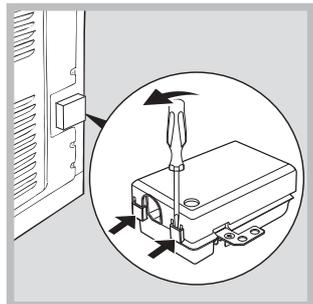
2. Install the power supply cable by loosening the cable clamp screw and the three wire contact screws L-N-
