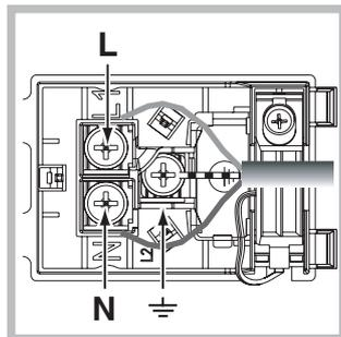
Connect the wires to the corresponding terminals: the Blue wire to the terminal marked (N), the Brown wire to the terminal marked (L) and the Yellow/Green wire to the terminal marked
