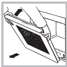
3. Grip the door on the two outer sides and close it approximately half way. Pull the door towards you, lifting it out of its seat (*see diagram*). To replace the door, reverse this sequence.
